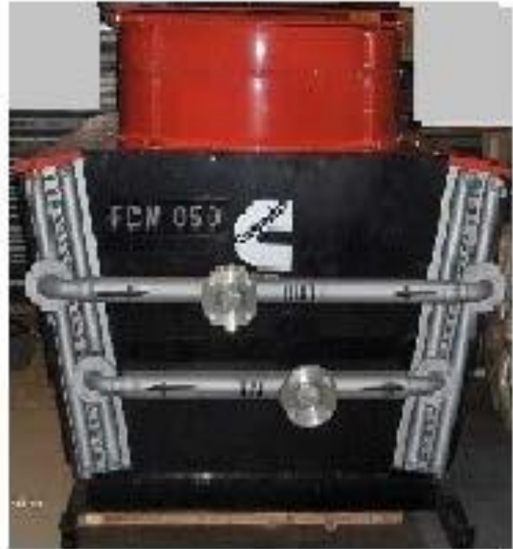
Remote radiator for Secondary circuit
